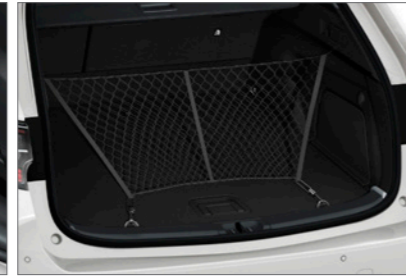
3 | Cargo Net - Vertical For complete installation, both Cargo Net - Vertical and Fitting kit for Cargo Net - Vertical (x2) are required. Part No. 99002-54Z00-002
