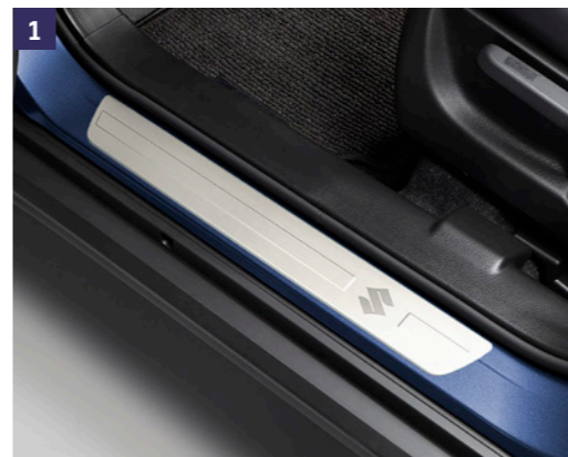
1 | Side Sill Scuff Aluminium, with S logo, four-piece set Part No. 990E0-61M60-001
